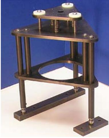
**Fig 3 Skeletal CLAMP Device Docked into Docking Features**
