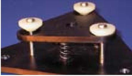
**Fig 5 Actual Top Mounting Plate Compliance Device**
