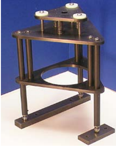
Fig 3 Skeletal CLAMP Device Docked into Docking Features
