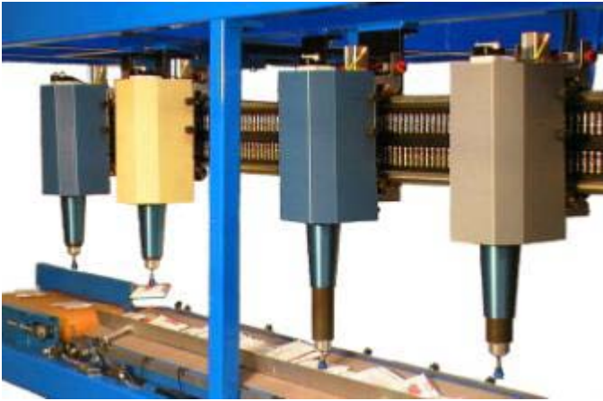
Fig. 4. Actual Trackbot tm material handling system. This application is using suction cups to singulate filled pouches. Multiple pouches are randomly located on the input conveyor, while 2 singulated pouches have been placed on the output conveyor at the left.
