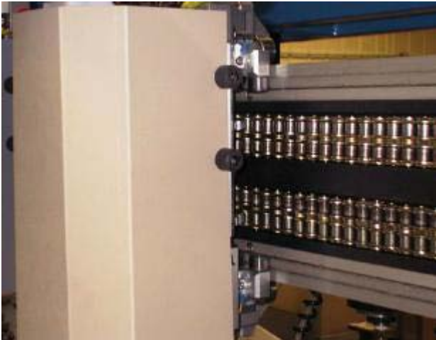
Fig. 5. Actual Trackbot rail and chain drive system. The upper and lower rails constrain the Bots. The lower chain moves and is used to propel the Bots. The upper chain is used for breaking and linear path position feedback.
