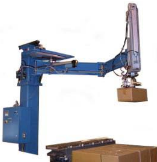
Fig. 3 Case palletizer [8] lifts boxes with flexible suction cups (Stackbot(tm))
