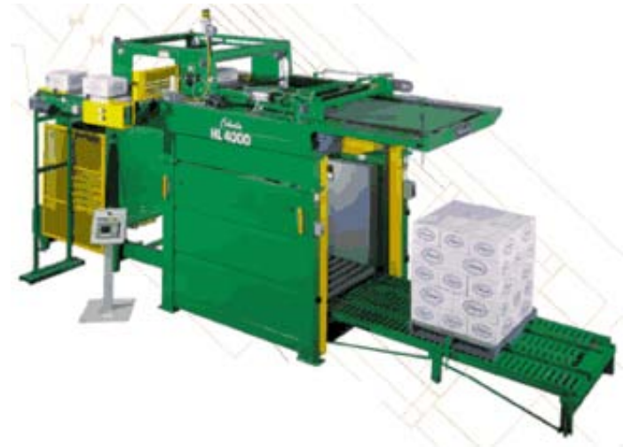
Fig. 4 Palletizer machine [7] forms an entire layer, then deposits it on a pallet (Columbia)
