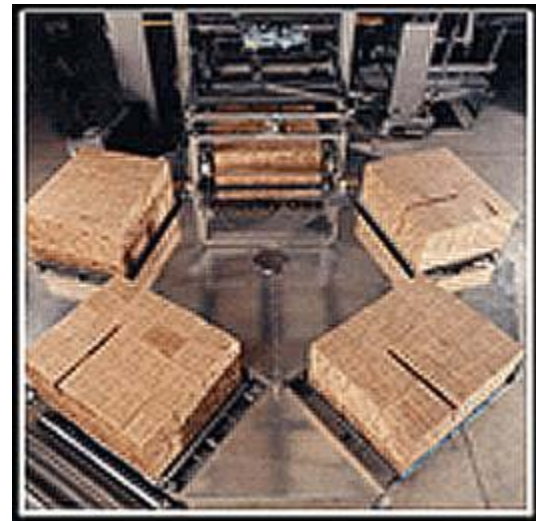
Fig. 5 Rotary palletizer [6] services multiple pallets (Priority One)
