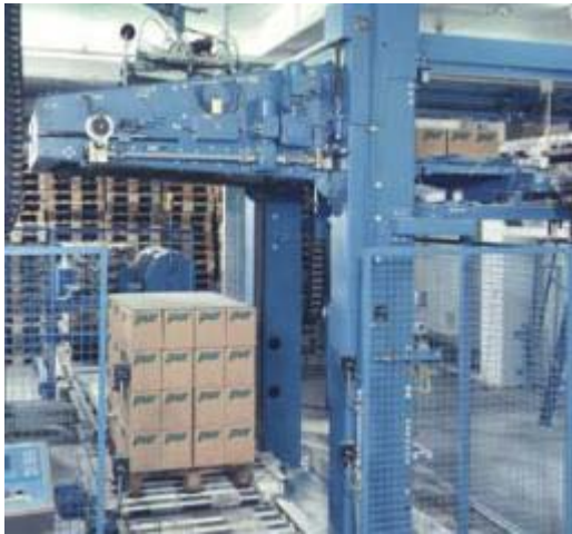
Fig. 6 High-speed Palletizer [5] has high-level infeed or input conveyor (Kettner)
