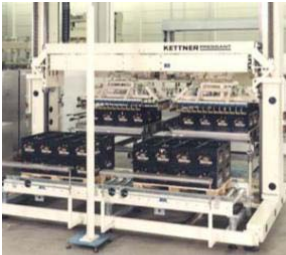
Fig. 7 Dual palletizer [5] has two pallet loading areas (Kettner)
