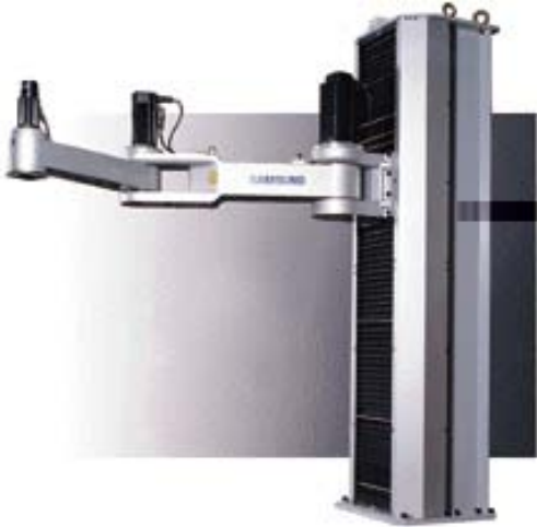
Fig. 2 4-axis palletizing robot [4] handles heavy payloads (Samsung)
