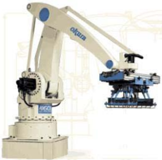
Fig. 1 Palletizing robot (7) fits into tight spaces while maximizing work envelope (Columbia/Okura)
